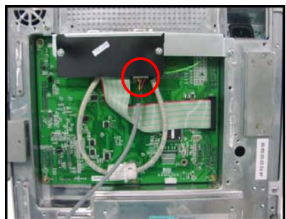
7. Connect WLAN kit wire to I/F BD of CN7. (Ensure must be connect properly)
