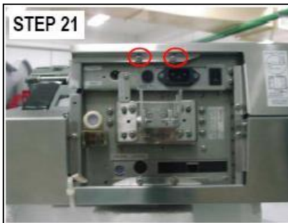
21. Tighten the screw (Red Circle) as shown.
