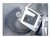
A look in the blade box shows a thin blade for a precise cut.
